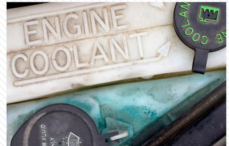
**Step 5** If your car doesn't have a reservoir for Antifreeze/Coolant, pour the fluid directly into your radiator. Again, be careful not to overflow.
